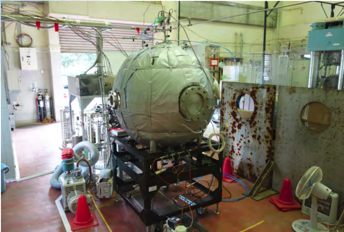
\Phi 100cm spherical combustion vessel equipped with mantle heater jacket
