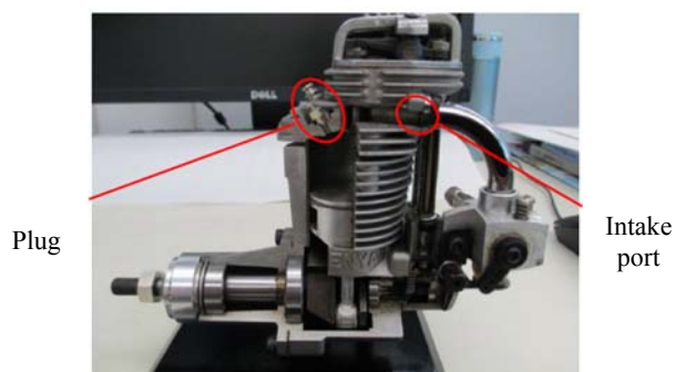
Fig. 3.6.2 Cut model of engine
