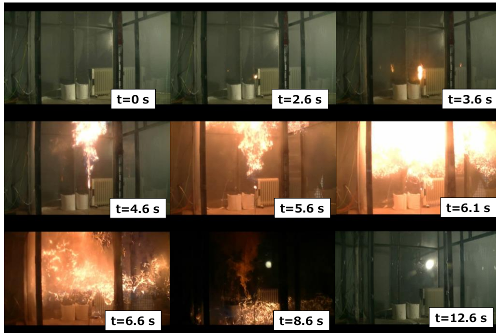
Figure 3-62: Sequence photos of the A2L refrigerant flame propagation without mechanical ventilation. Variable t: time since Ni-Cr wire coil was energized, Refrigerant: R1234ze(E), Leak amount: UFL (5.7 kg).
