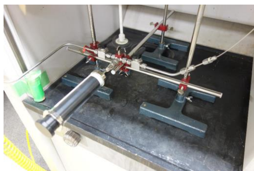
Figure 4-14 ASTM E659 test equipment (left: plunger system, right: test flask with copper foil).
