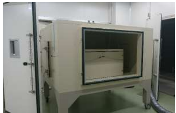
Fig.3.4.2-4 Appearance of indoor unit wind chamber
