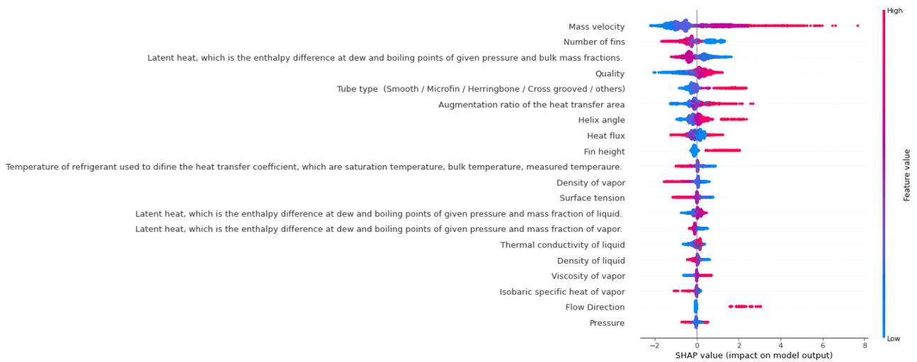
Fig.3.1.4-22 SHAP values of transfer learning model of heat transfer coefficient (Model 6)
