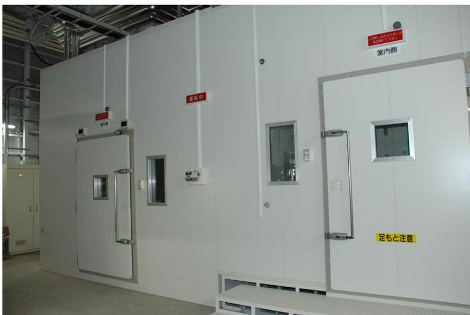
Fig. 3-1 Calorie meter, outdoor unit test room (left), and indoor unit test room (right)
