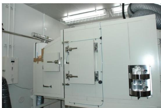
Fig. 3-4 Wind receiving chamber in the indoor unit test room
