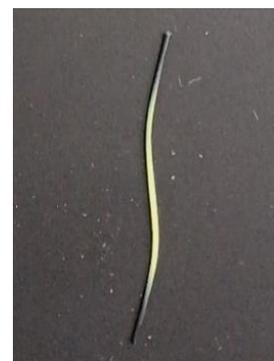
Fig.3-46 Photo of tungsten wire after being used for the ignition test.
