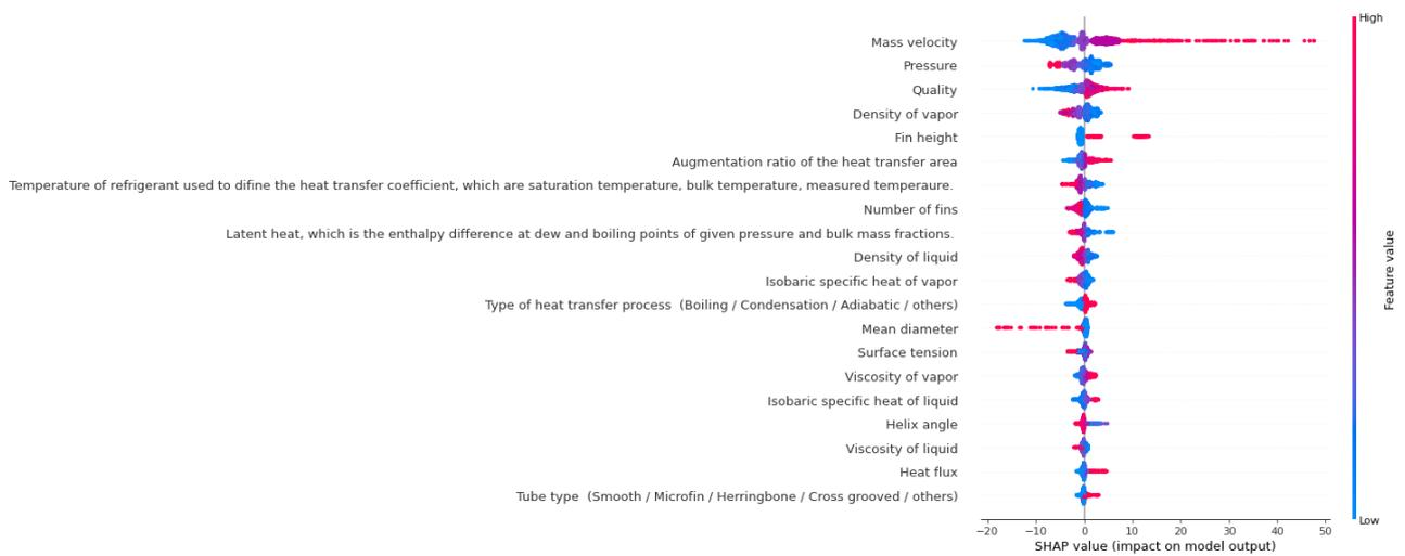
Fig.3.1.4-23 SHAP values of DNN of pressure drop (Model 4)
