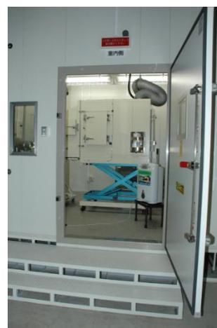
Fig. 3-3 Indoor unit test room
