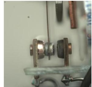
Fig.3-12 Photo of the electric contact after conducting the ignition test.
