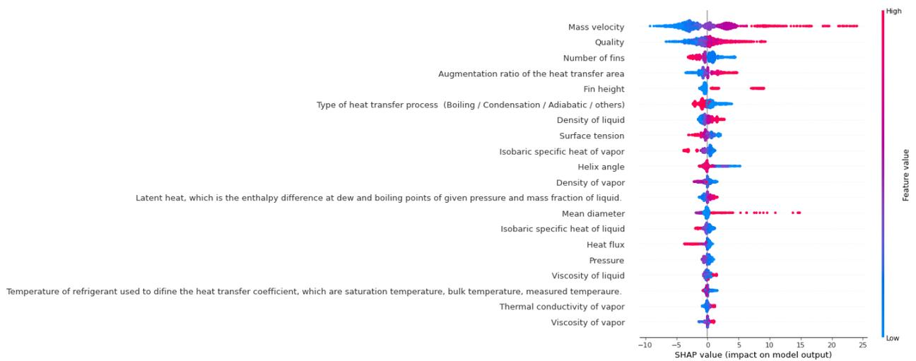
Fig.3.1.4-24 SHAP values of fine-tuning model of pressure drop (Model 2)
