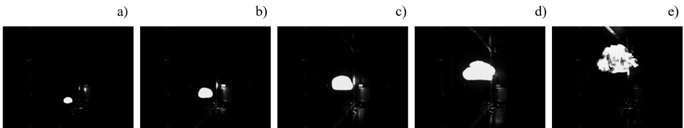
Fig. 4-5-2 Fire observed after ignition at 2 min after finishing discharge. (R1234yf, 100 ms each)
