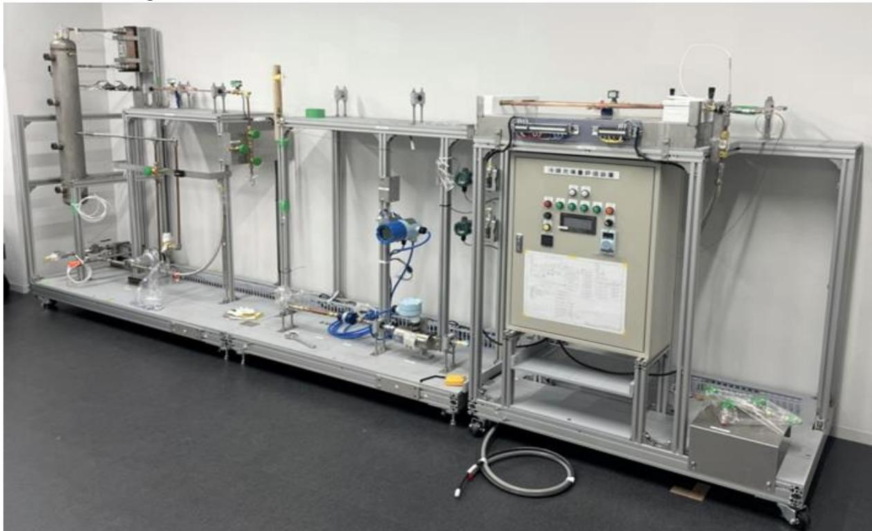
Fig.3.1.5-15 External view of refrigerant filling amount evaluation device
