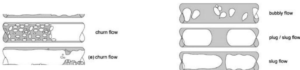
Fig.3.1.5-11 Various flow pattern of two-phase flow in microchannel
