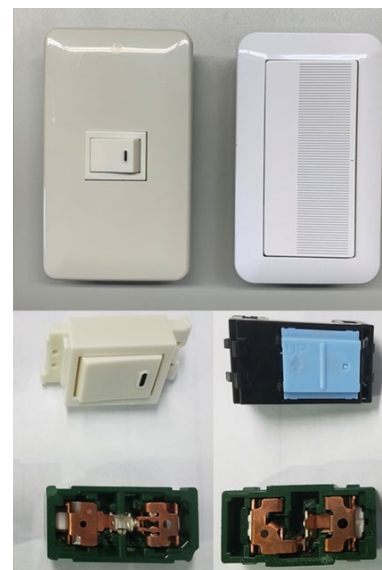
Fig. 3-7 Photos of test switches for lighting. Upper: Body Middle: Button Low: Electrical contacts Left: Type A, Right: Type B
